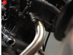
If the exhaust gasket has stayed on the engine, remove it now as it's not required with the Scorpion system.
