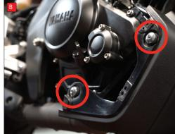
A) Remove the 3 screws on the right side lower front panel and then the 3 on the left side as well.
